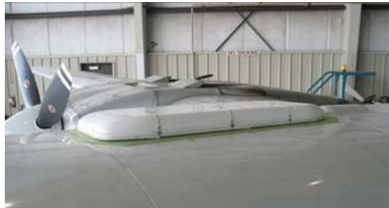
FIGURE 25 - Satellite Communication System Phased Array Antenna
